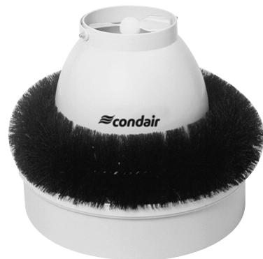
This filter brush is fixed to an aluminium ring, which can be put into the water reservoir (see figure above). The electric flex of the appliance must be drawn through the ring. The air required by the unit is then forced to pass through the filter brush, which traps the fibrous dust. This prevents the accumulation of dirt in the unit to a large extent, and maintenance can be carried out at correspondingly longer intervals.
