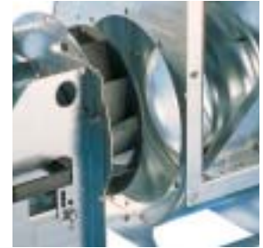
GTHB-1 features an easy removal of the impeller for cleaning purposes.
